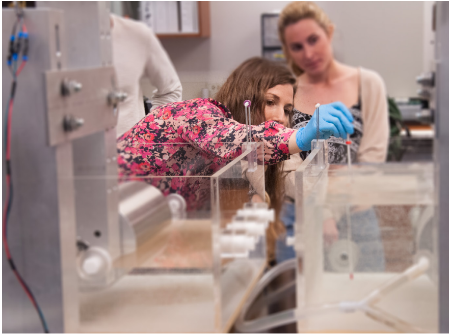
L to R: NM Tech undergrad Cassandra Sanchez makes adjustments as she fabricates hollow fiber membranes; Hollow fiber membranes encased in fiberglass and ready for lab deployment.
