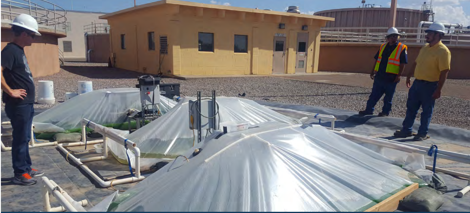
Dr. Omar Holgin (far right) checks on his team's algal wastewater treatment testbed
