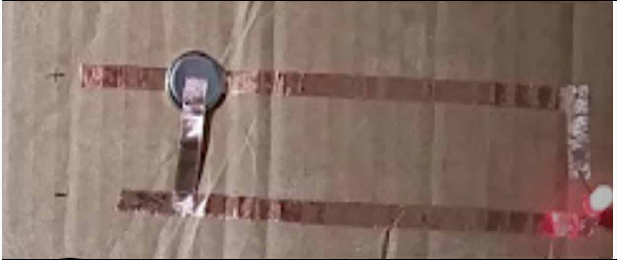
Figure 3: Picture of the experimental setup for circuit design with maker tape in Lesson 2.
