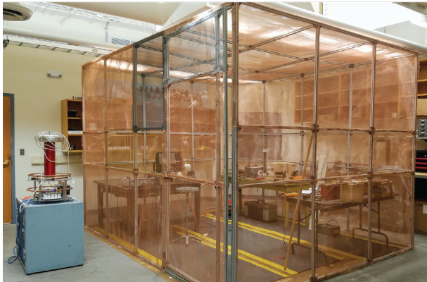
Figure 1 - The newly developed Langmuir Spark Lab. (a) Faraday cage. (b) First experiment.
